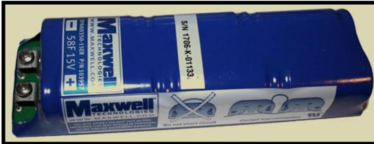
Another component that will be replacing some lead-acid batteries on powersports vehicles in the near future is the ultracapacitor. Ultracapacitors are very lightweight and can deliver
